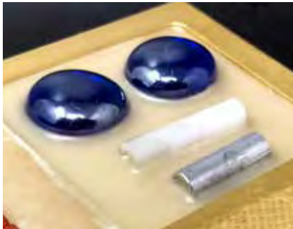
The stick form material can be used in shallow cavities for holding concave and convex pieces. It will also stabilize delicate parts during machining.
