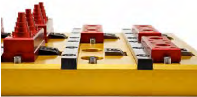
Locating rails are made of low carbon steel and are precision ground square. They are available in a number of sizes and lengths to suit most applications.
