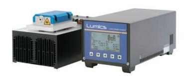
Lumics provides high precision and cost effective power supplies and drivers for 14pin butterfly, TO220 and Ludcean<sup>TM</sup> Mini 4 series laser. Standard interfaces are the RS232 port, and analog current control. You can set arbitrary limits for current, voltage and laser diode heat sink temperature. The device can modulate the laser internally by on-board oscillator or may be configured for external modulation. Multiple circuits watch over the laser security to avoid any harm to the laser.
