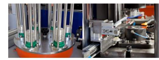
Standard feeding system from the 6-fold blanks magazine located at the side of the press, the blanks are taken by vacuum cups and placed to the coining tool.
