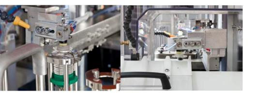
Both sides of coins / bars are cleaned with dried cleaned air in different moment of the handling. Air stream is adjustable.
