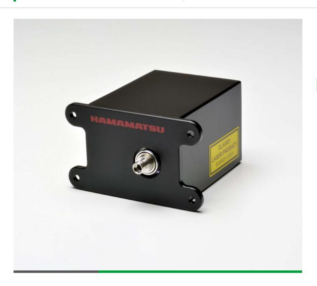
The Fourier transform infrared spectrometer (FTIR) engine is compact enough to carry in just one hand. A Michelson optical interferometer and control circuit are built into a palm-sized case. Spectrum and absorbance can be measured by connecting a PC via USB.
