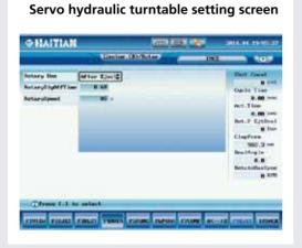
The control system of the servo hydraulic turntable is equipped with a rotating encoder, which provides immediate feedback on the turntable location. By changing the degree of opening of the turntable's proportional direction valve as well as the system's pressure and flow, the closed loop control is established.
