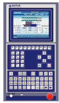
Control system especially for the multi component injection molding machines, with two CPU for the parallel processing of data
