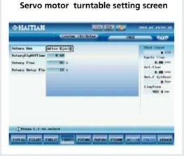
The servo motor turntable system is equipped with an electric servo motor and inverter, to feedback on the turntable position, by changing the speed and torsion of the electric servo motor, the closed loop control is established. The servo motor electrical turntables has got the advantage of speed, stability and precision
