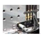
Convenient interfaces for mold auxiliary connections
