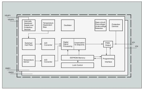
Fig. 1: Block diagram of the HAR 2425 with ratiometric analog output
