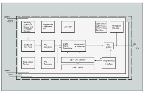
Fig. 2: Block diagram of the HAR 2455 with PWM output
