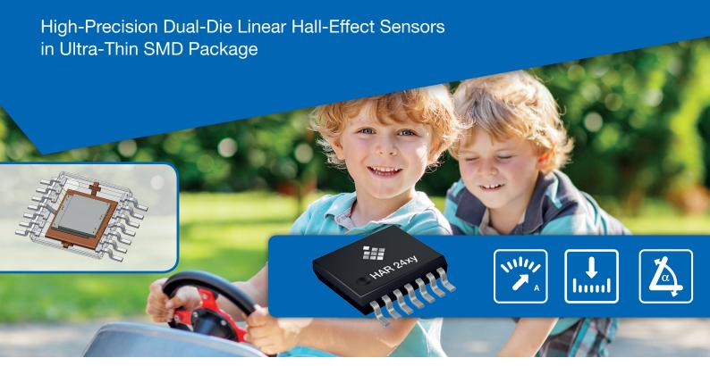
HAR 24xy is a dual-die programmable linear Hall-effect sensor family available in the TSSOP14 package with a package height of less than 1 mm. Each sensor provides true redundancy as it consists of two independent dies stacked in a single package. The stacked-die architecture ensures that both dies occupy the same magnetic field position, thus generating synchronous measurement outputs.
