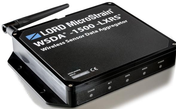
WSDA<sup>®</sup>-1500-LXRS<sup>®</sup> - network-ready gateway for high-speed, sophisticated data aggregation, with J1939 CAN and Ethernet interfaces
