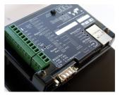
Convenient pluggable screw terminal connections for plant terminations.
