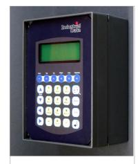
The WMX wall mount enclosure comprises 2 sections with an "O" ring seal to preserve IP65 ingress protection. The EELX fits to the front part permitting the rear section to be installed separately. The material is ABS. Used together with the HP overlay and sealing gasket for a complete weatherproof solution suitable for outdoor installation
