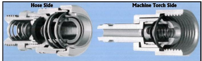
The high quality reverse - flow valve helps to prevent the possibility of gases mixing. When a backfire occurs it shuts off pressure to the torch.
