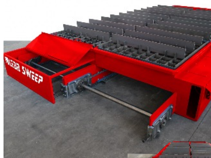
Dual sweeper: From 10 - 24 ft. cutting width. (rear idler shaft shown in picture above)
