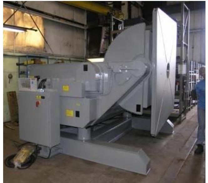
GE500VF, Rack and Pinion Elevation rated at 50,000 Lbs. Capacity
