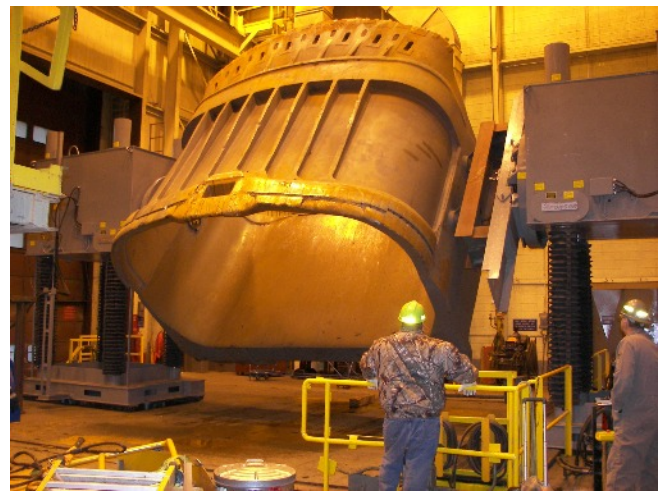
160,000 lb Elevating HTS for Mining Shovel Repair
