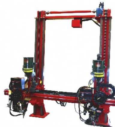
Pantograph Welding Gantry
