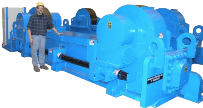
1,000 MT Roll Set for Heavy-walled Nuclear Vessels
