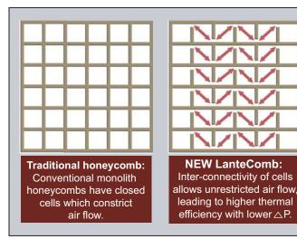
LanteComb is a technological breakthrough in structured heat recovery media for RTOs.
