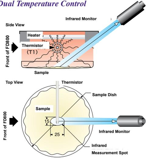
In addition to the ambient temperature in the drying chamber (T1), the FD800 monitors sample temperature (T2) (Patent pending), providing unsurpassed drying control, resulting in optimized drying times, and minimizing or eliminating sample degradation and resulting measurement accuracy.
