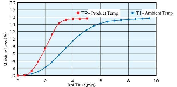
Sample Surface Temperature: Starting with a high temperature, (T2) efficiently conducts heat drying
