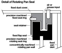
fixed flap seal also lies inside the seal ring joint. All rotating shafts that penetrate the dust cover are double sealed with grease or air purge between the seals. These features all combine to help eliminate any dust or material leakage from a Lancaster Mixer.
