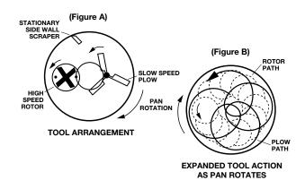
**FIGURE A** illustrates combined action of the pan rotating clockwise while the off-center mixing tool assemblies rotate counter-clockwise.
