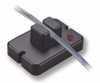
ntrotek BD8/BD9 Integral sensors combine BD3 electronics with a free-entry sensor head. Constructed of soft polyurethane, the BD8 is recommended for rigid tubing. The rigid epoxy or ABS plastic BD9 is recommended for flexible tubing.
