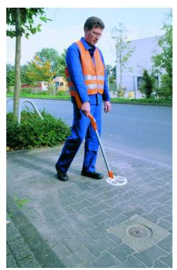
As a result of the downward-directed search field, the detector can be used in immediate proximity to metal fences or parked cars. The one hand held unit is designed for use by one hand only and offers optimal ergonomics for fatigue-free working.
