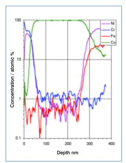
results in easy quantification of alloys and high concentration impurities, without the need of matrix matched reference materials.
