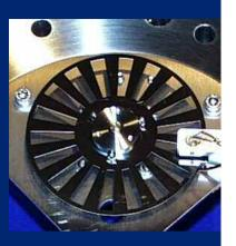
Integrated multibladed rotating disc chopper with UHV stepper motor drive and LED optodetector linked directly to MASsoft control software via on-board programmable signal gating module.
