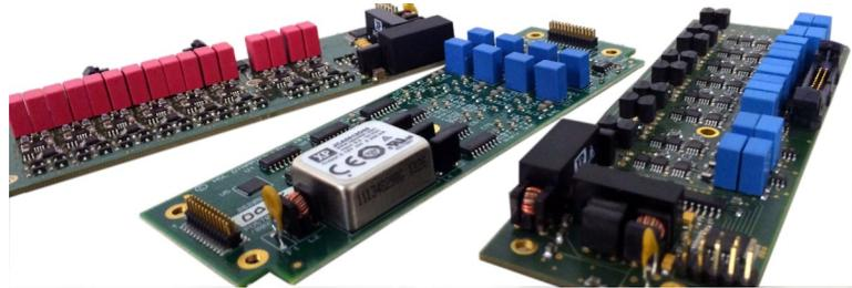
HGL has designed a set of conditioning cards that fulfil most industry standard requirements. However more cards are developed as clients' requirements change. The signal conditioning options currently available for the Dragonfly<sup>8</sup> module are:
