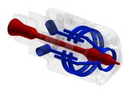
The pneumatically controlled nozzle type NE has a needle shut-off mechanism which stops the melt stream directly at the mold interface. Rubber, liquid silicone rubber and other elastomers can be processed without fear of premature vulcanization due to the nozzle's integrated cooling system, which uniquely regulates temperature through the entire nozzle. The nozzle can also be fitted with an interchangeable diving tip for cold channel applications.
