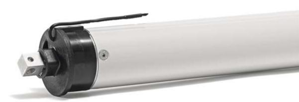
The Type 11 drives are available in 100 Nm and 120 Nm. The high precision mechanical limit switches are easily accessible and ensure a very high repetitive accuracy. The drive features a plug-able cable which is 2.0 m long.
