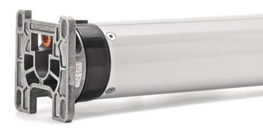
Type 15 is the ideal drive for heavy roller shutters, small rolling gates and roller grilles. These are characterized by the well-balanced torques, 120 Nm, 150 Nm, 180 Nm, 230 Nm and 300 Nm, each with 230V/50 Hz.
