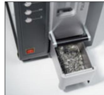
Comminution of ferrous alloys with the Jaw Crusher PULVERISETTE 1 premium line – 6.5 mm gap width
