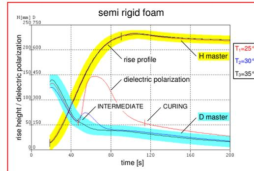
Fig. 3: The figure shows the variation of the dielectric polarization of a semi rigid formulation at three different temperatures. The H master and the D master are generated by the software FOAM for QC purposes.
