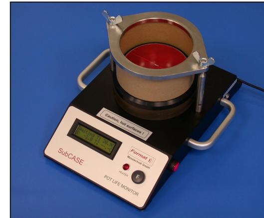
Fig. 4: The temperature controlled curing monitor device SubCASE® measures the pot life and the curing of Coatings, Adhesives, Sealants and Elastomers (CASE).
