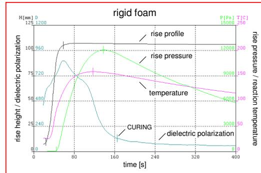
Fig. 2: The experimental data for rise height, dielectric polarization, rise pressure and temperature of a rigid foam formulation. The dielectric polarization was measured at low frequency, revealing perfectly the curing of the formulation.
