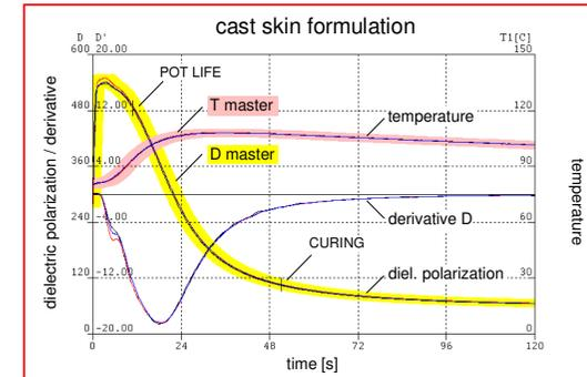
Fig. 5: Three dielectric polarization and temperature measurements of a transparent, fast curing cast skin formulation, which is used for fine wood decoration. The data show perfect reproducibility.
