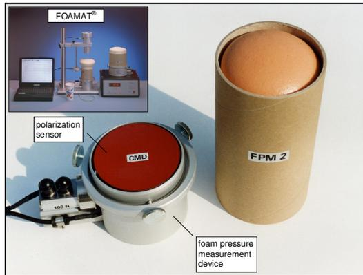
Fig. 1: The polarization sensor CMD2, integrated into the foam pressure measurement device FPM2, measures the dielectric polarization of the foam in combination with rise profile and temperature.
