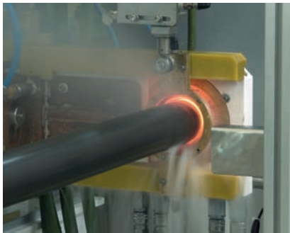
Customized installation for hardening and tempering of drilling pipes
