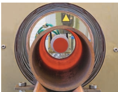
Stress relief of oil and gas pipe
