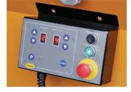
\*Digital panel can be turned off at any time with machine reverting to a single angle preset system If the panel fails or is unneccesary for the job, you can still bend with full control and accuracy.
