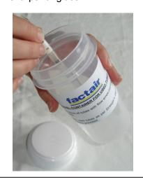
Ensure the oil tube is kept vertical throughout this process
