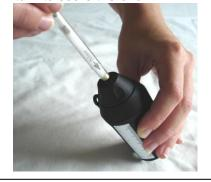
2. Push the tube at an angle to break the tip.
