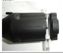
5. With one hand holding the cutter and the other holding the tube. With your thumb against the base of the cutter, apply pressure to the tube. This should break the inner tube.
