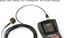
vibration to ISO 2631, as well as vibration on passenger and merchant ships to ISO 6954.
