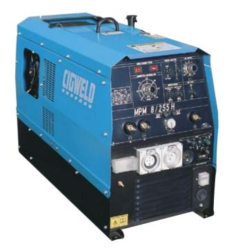
The CIGWELD MPM 8/255H is a petrol powered welding machine that is driven by an ultra reliable 18HP HONDA® engine, which delivers a maximum welding output of 255 amps. With its multi process capabilities, this unit performs exceptionally in a range of welding applications including MMAW(Stick), GMAW (MIG) and GTAW (TIG) the unit provides both 8 kVA three phase and 7 kVA single phase auxiliary power.
