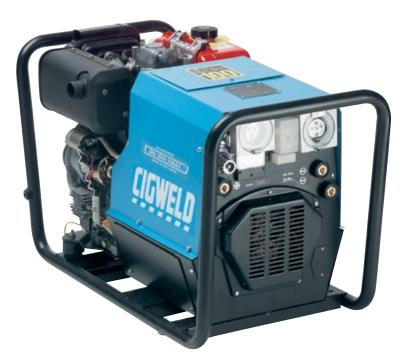
The CIGWELD MPM 5/170Y is a diesel engine driven welding power source, which has the flexibility of an electric or manual start. With its patented asynchronous alternator design it delivers an ultra smooth welding output and guarantees high efficiency, reduced maintenance and an extended machine life.
