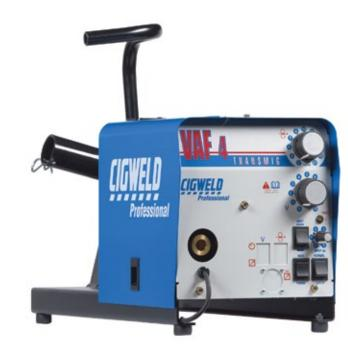
The VAF-4 Professional 4 Roll Wire Feeder is compact, light weight and easy to use wire feeder that is suitable for use on a broad range of power sources. The unit incorporates a range of features including wire inching, gas purge, trigger latching, along with standard features such as wirespeed control and spot timer control.
