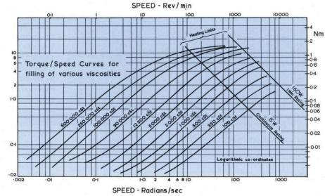
The Q-CRD continuous rotation dashpot has a fixed rate performance and is complementary to the larger adjustable rate S-CRD and T-CRD. It proves to be economical where use of the other models may not be justified.
