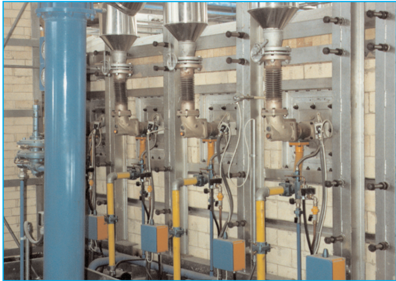
Rocking frit melting furnace for pre-heated air (450° C), "Nozzle Mix" burners (Poppi Eurotech)
