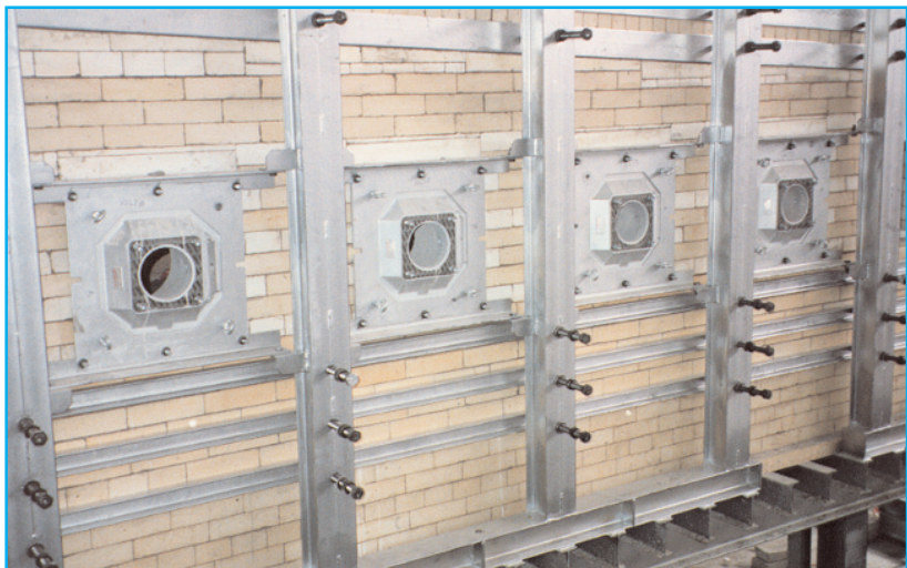
Rocking frit melting furnace for pre-heated air (450° C), "Nozzle Mix" burners (Poppi Eurotech)
