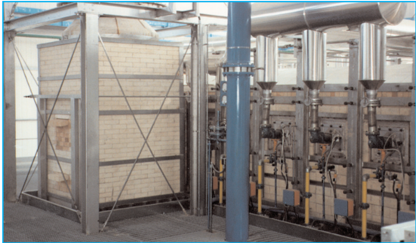
Rocking frit melting furnace for pre-heated air (450° C), "Nozzle Mix" burners (Poppi Eurotech)
