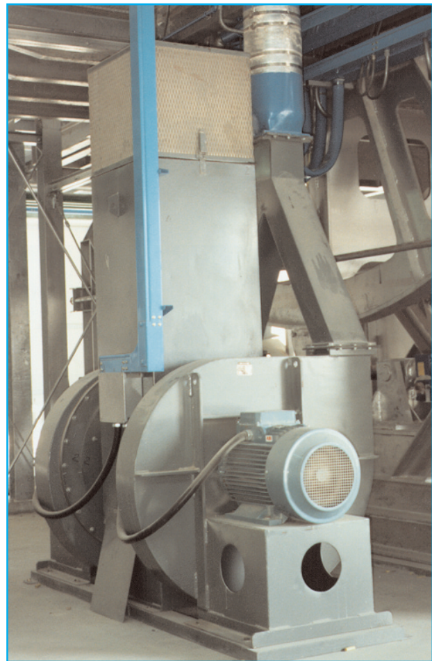
Rocking frit melting furnace for pre-heated air (450° C), "Nozzle Mix" burners Pre- assembled, comburent air blowing group (Poppi Eurotech)
