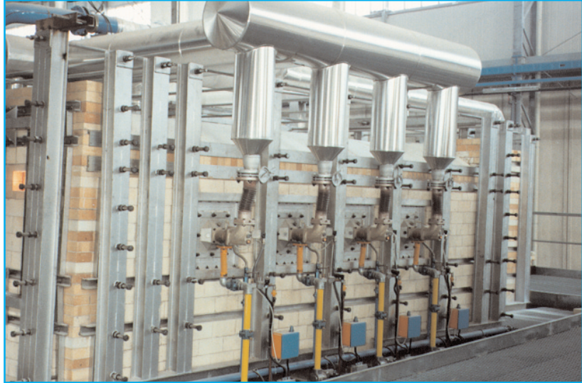
Rocking frit melting furnace for pre-heated air (450° C), "Nozzle Mix" burners (Poppi Eurotech)
