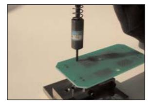
Place male connector into lower tool, with its termination side facing upwards, and place manual device on signal contact.
