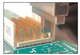
Press in the signal contact. The manual press-fitting device is guided through the shield of the signal contact.
