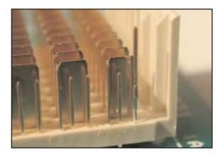
Fit new contact. The alignment of the contact should be noted. Align the contact such that it fits into the rectangular aperture in the housing.
