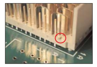
Clean position on male connector housing (e.g. with a pair of pincers). As plastic residues may remain when the contact is pressed out.
