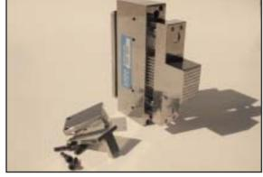
Adjustment with the arrester device screwed off. For pressing out male connectors where the signal contacts do protrude from the printed circuit board.
