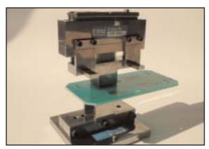
Clamp the lower and upper tool into the press. Then press out the complete male connector in a downward direction. The upper tool can be adjusted variously depending on the thickness of the printed circuit board or the pin termination length. Warning: Row 1 is marked.
