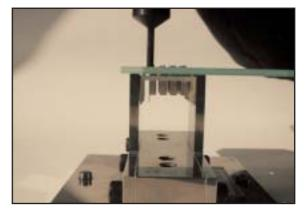
Use manual device to press out and remove signal contact in a downward direction.
