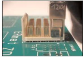
By pressing with the manual device, the contact is pressed in above the contact tip. (Manual device is different depending on the contact length)
