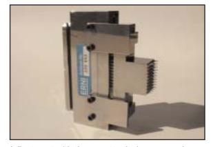
Adjustment with the arrester device screwed on. For pressing out male connectors where the signal contacts do not protrude from the printed circuit board.
