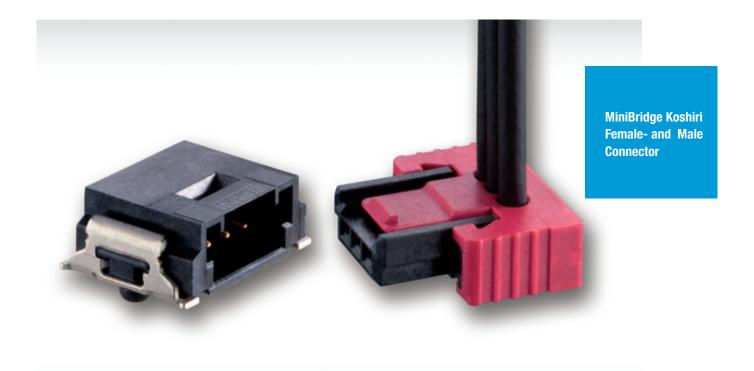
The single row MiniBridge connector Koshiri version with a 1.27 mm pitch offers very high level of mating reliability. The housing geometry avoids damage of the male contacts even in case of improper skewed insertion.
