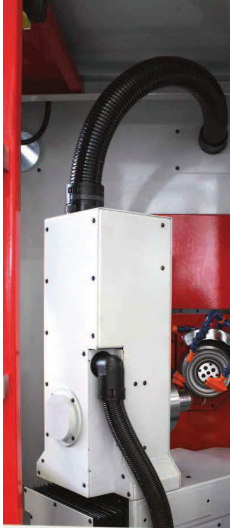
Automatic steady rest and tailstock for production and regrinding small tools (optional)
