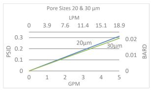
Flow rates for Cartridge filters are per 10-inch length. The test fluid is water at ambient temperature.
