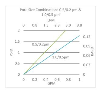
Flow rates for Capsule filters are per square foot of membrane area. The test fluid is water at ambient temperature. Flows are tested using a 2" capsule filter with ½" FNPT inlet and outlet ports. Rates will vary based on end configuration of the capsule.
