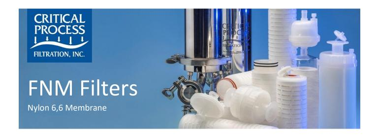
FNM cartridge and capsule filters are constructed with long-proven, absolute rated, Nylon 6,6 membrane. Designed to comply will all FDA requirements for the food industry, these high purity filters are used for removing organisms in nonfermenting liquids, sterilizing of aseptically packaged products and cleaning water. Pore sizes range from 0.10 to 0.65  $\mu m$  and the filter sizes scale from laboratory to full production using identical materials to ensure consistent results.
