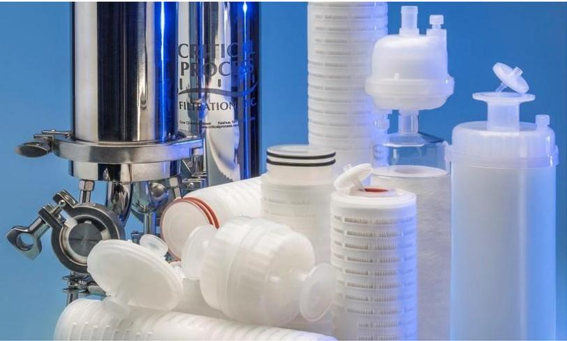
BPS filters offer single and dual layer Polyethersulfone (PES) cartridge and capsule filters for use with aqueous liquids. Pore sizes range from 0.03 to 1.2  $\mu\text{m}$  and filter sizes scale from laboratory to full production using identical materials to ensure consistent results.
