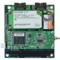
Janus-MM with GPS and Wireless modem Modules Installed
