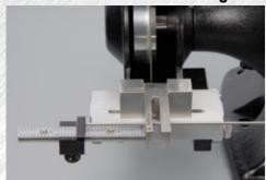
Produces smooth diamond cut electrodes on a selectable length scale.
