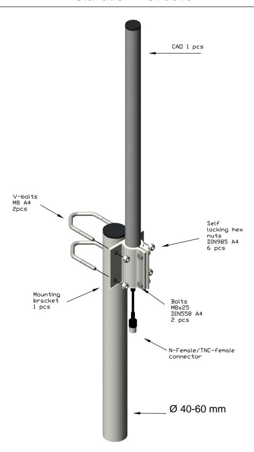
For proper weather protection all connectors and cable junctions should be covered by self-amalgamating tape or equivalent
