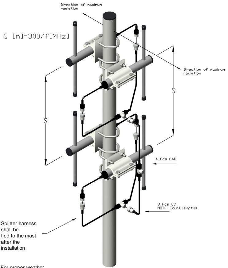
For proper weather protection all connectors and cable junctions should be covered by self-amalgamating tape or equivalent
