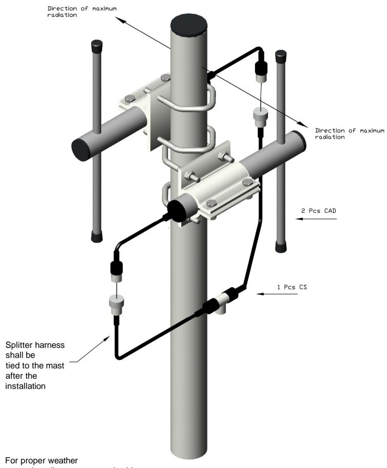
protection all connectors and cable junctions should be covered by self-amalgamating tape or equivalent
