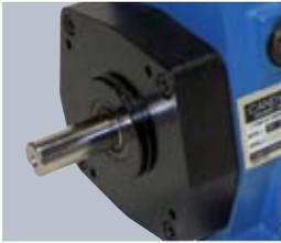
Standard units are shipped with a control knob for manual phase adjustments. The control shaft, a keyed shaft extension, may be ordered as an option and installed in place of the standard knob. The control shaft may then be used to mount a control motor or flexible shaft assembly. The control shaft may be installed on the knob side, the lock side, or on both sides of the Differential.
