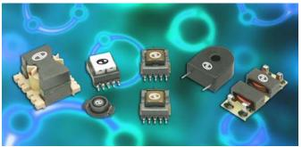
The most common magnetics components found in power supply designs include: switcher transformers, gate drive transformers, current sense transformers, inductors and dual planar inductors.
