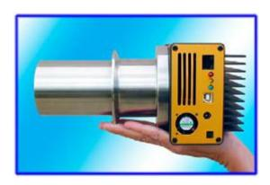
The user has a choice of several different detectors, both silicon and InGaAs. Silicon diode arrays and CCDs cover the visible range, from 380nm to 1100nm. InGaAs detectors provide coverage from 900nm to 2200nm.
