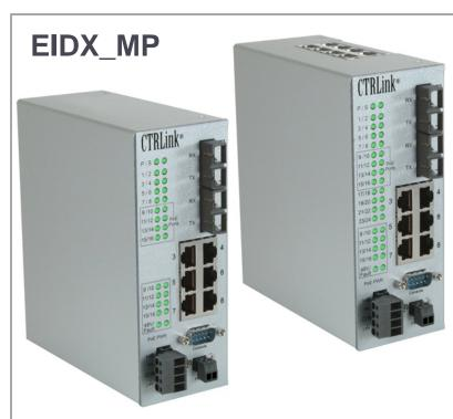
Two-port single-mode and multimode fibre optic versions are available with ST and SC connectors.
