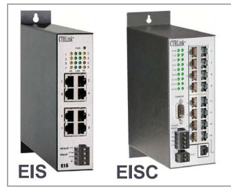
The VLAN feature in the EISC16 was used to isolate broadcast messages to only those stations of interest.
