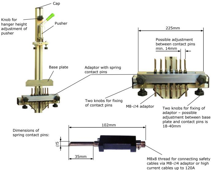
Continuous current: 100A Maximum current: 120A 10min./1h Pin resistance: 0.6m0@100A (resistance bel
