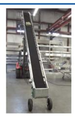
Made out of lightweight T6-6061 aluminum for easy assembly and portability
