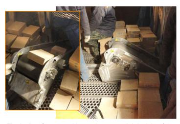
The Incline Conveyor drive end mounts slightly right of the center of the bricking machine platform with guide pegs that slip through the decking of the work platform.
