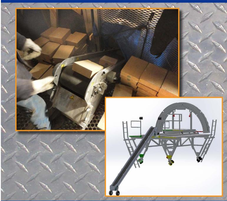
All-aluminum, modular conveyor system designed to easily transport brick from kiln floor to bricking machine work platform
