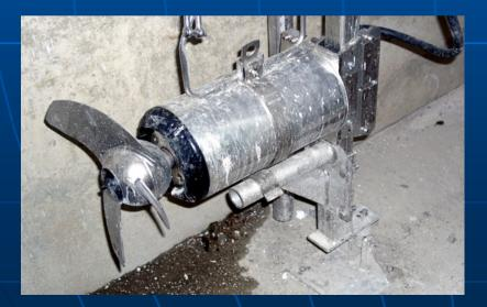
Low speed submersed propeller mixers
