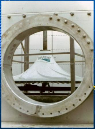
Low speed and "soft" energy input do not destroy flakes (in contrary to high speed submersed mixers)
